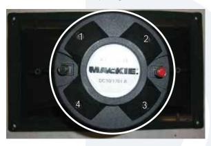
The horn assembly is shown above with the high frequency driver circled. Four screws need to be removed from the driver using the 3mm allen wrench.
